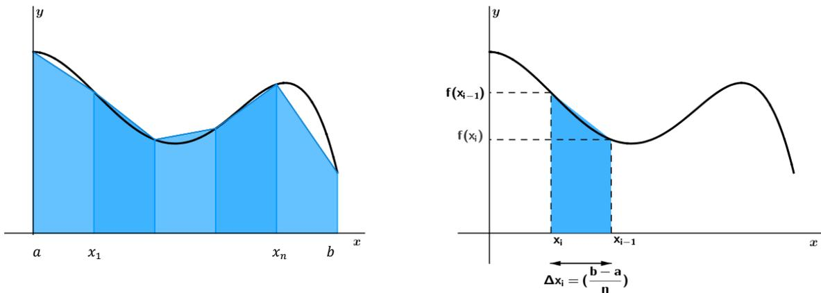
$$\begin{aligned} \int_a^b f(x) dx &\cong \frac{(b-a)}{2n} (f(a) + 2f(x_1) + \dots + 2f(x_{n-2}) + 2f(x_{n-1}) + f(b)) = \\ &\int_a^b f(x) dx \cong \Delta x \left( \frac{E}{2} + P + I \right) \end{aligned}$$
