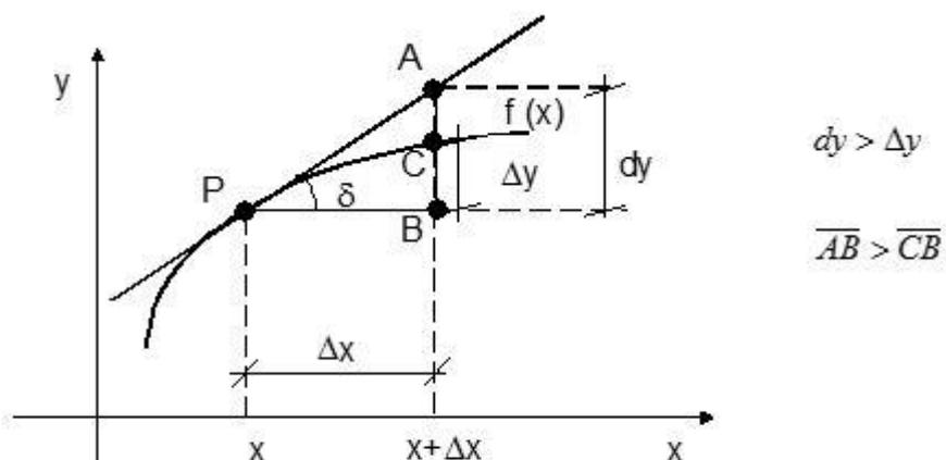
$$\operatorname{tg} \delta = \frac{\overline{AB}}{\Delta x} = f'(x) \therefore \overline{AB} = f'(x) \Delta x = dy \therefore dy = \overline{AB}$$
