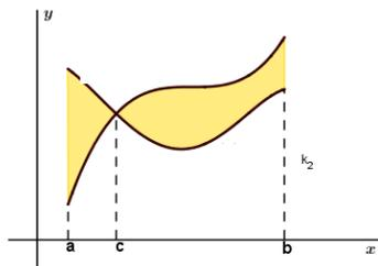
$$\text{Área} = \int_a^c (f(x) - g(x)) \, dx + \int_c^b (g(x) - f(x)) \, dx$$
