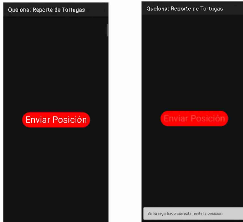
(a) Single screen fishermen application. In (b) Single screen of fishermen application, order to maintain the simplicity of the system, only one button was tested to record the position in which the angler encountered a turtle. The button is disabled for 20 seconds after successfully registering the location.
